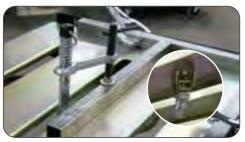
The MagSpring<sup>™</sup> Clamps can be inserted into the 1.1 slots on the Nomad™ Tabletop for hold down clamping. Magnetic V-Pad jaw holds underneath the table to keep the clamp in the up-right, "ready to use" position.
