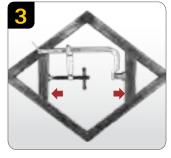
Spreader Reverse the clamp arm and create a Spreader Clamp.
