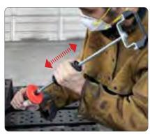
The built-in sliding hammer enables odd direction/position hammering.
