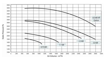
MJC Mini range fan performance, with open outlet, at running speed 2900/min.
